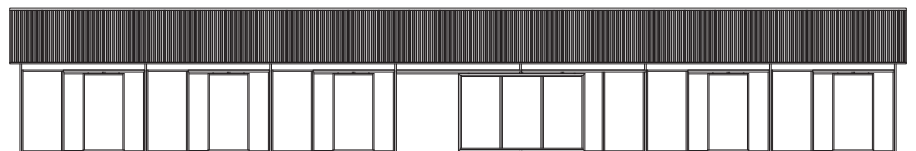
Side Elevation Showing 12' Side Breezeway Door Half Open (Shown with 4' Rear Doors Half Open)
